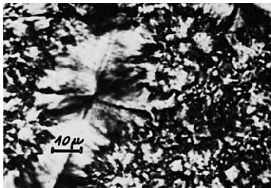
Fig. 4. Spherulitic structure, PCL.
